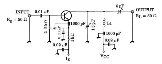
$L_1$ : 0.8 mm $\phi$  silver plated copper wire, 4 turns. 10 mm ID, 8 mm length.
