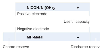
FIG. 3 Schematic representation of the electrodes, demonstrating useful capacity, charge reserve and discharge reserve
