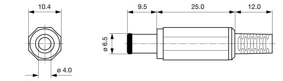
Cable diameter max. 4.0 mm
