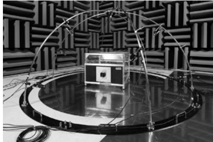
Noise characteristic measurement equipment
