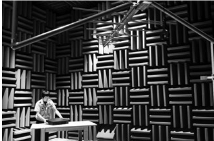
Acoustic radio wave anechoic chamber
