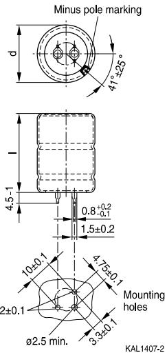
Snap-in capacitors are available with 3 terminals (length (4.5 –1) mm). PET insulation is marked with label "PET" on the sleeve.
