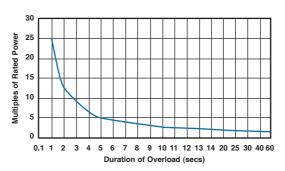
This graph indicates the amount that the rated power (at 20°C) of the standard HS Series resistor may be increased for overloads of 100mS to 60S
