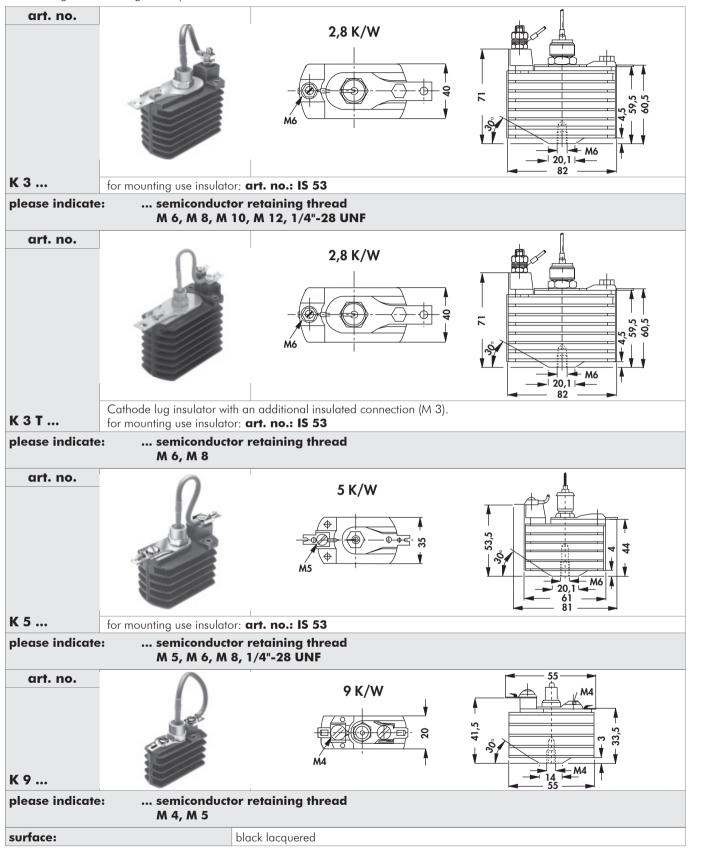
Mounting for TO 3 angle Order example Standard aluminium profiles **Heatsinks for PCB**
