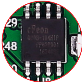
Figure 11-1: Flash memory module
