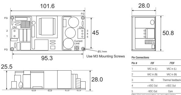
Filter Ground connection via mounting holes Dimension Tolerance  $\pm$  0.25 mm
