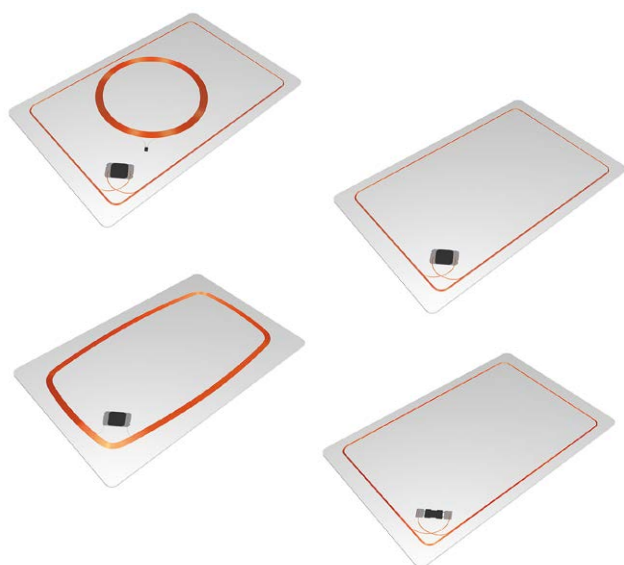
The pictures demonstrate different options how to position one or two contactless technologies in one card.
