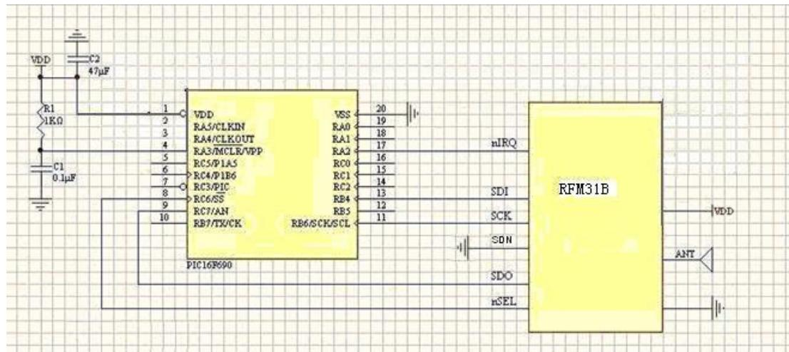
Note: The SDN pin connect to GND or control by IO port of MCU. When the module is in working, the SDN pin must set to low. When the SDN pin is high, the Module current consumption is 0.01uA.
