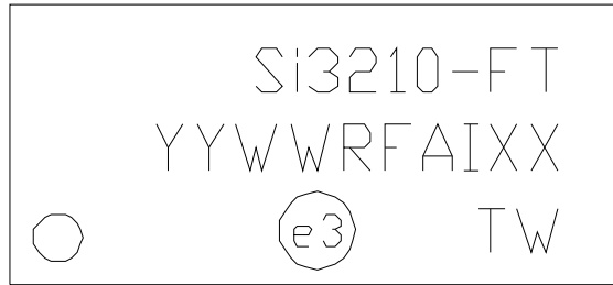
Figure 40. TSSOP Top Mark Diagram
