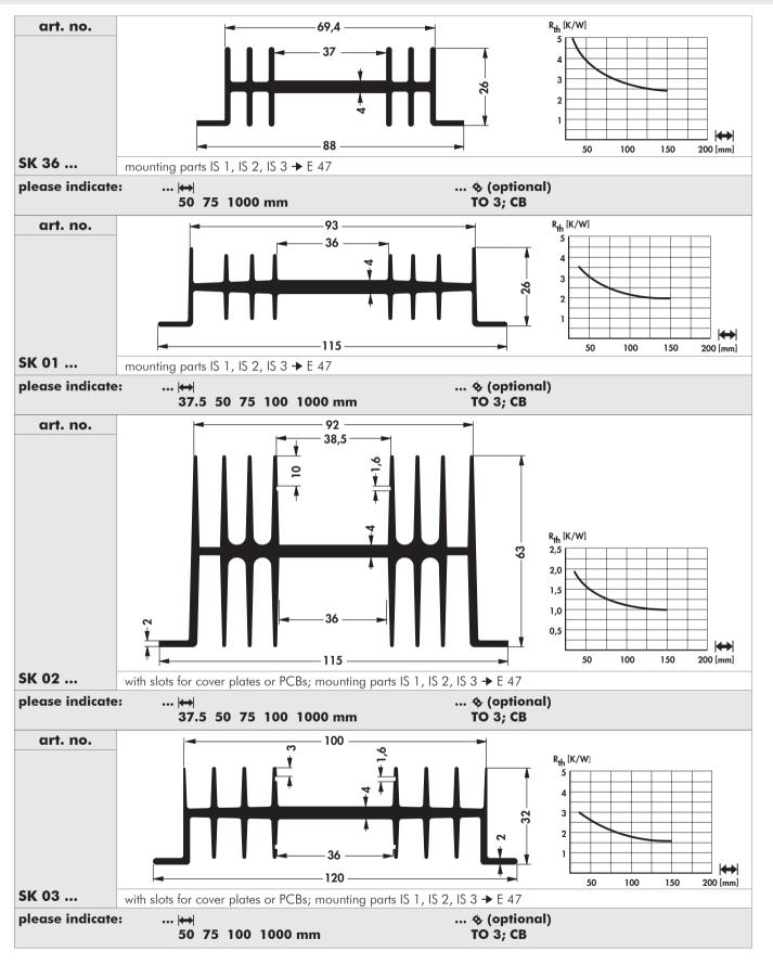
Heatsinks for Solid State Relay Heatsink special design Special profiles Technical introduction  $\begin{array}{l} \rightarrow \quad A \ 11 - 12 \\ \rightarrow \quad A \ 135 - 136 \\ \rightarrow \quad A \ 138 \\ \rightarrow \quad A \ 2 - 7 \end{array}$
