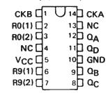
SN5492A, SN54LS92 . . . J OR W PACKAGE SN7492A . . . N PACKAGE SN74LS92 . . . D OR N PACKAGE (TOP VIEW)
