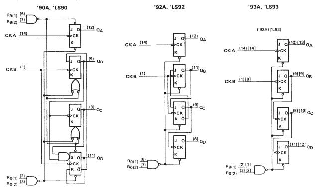
The J and K inputs shown without connection are for reference only and are functionally at a high level. Pin numbers shown in () are for the 'LS93 and '93A and pin numbers shown in () are for the 54L93.
