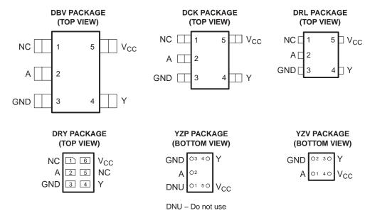
NC – No internal connection See mechanical drawings for dimensions.
