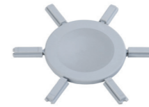
Coding Star CS2-5.0/5.08-LIGHT GREY-HT Article Number: 50000000028 The tongues of the reflowable coding star are inserted into the coding slits to prevent the multi-connector from being plugged in incorrectly. This coding star is usable in reflow soldering processes.
