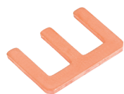
Brücke, 3-polig, BR/3-3.5/3.81-L4.7 Article Number: 50000000014 Uninsulated bridge for multi-connection. Can be used for terminal blocks and multi-connectors with spacing 3.5 mm and 3.81 mm.
