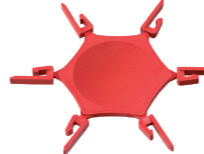
Coding Star CS3-5.0/5.08-RED Article Number: 50000000025 The tongues of the coding star are inserted into the coding slits of the terminal block to prevent the multi-connector from being plugged in incorrectly.
