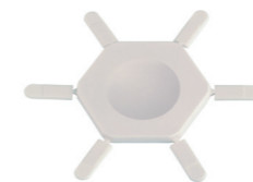
Coding Star CS1-3.5/3.81-NATURAL-HT Article Number: 50000000022 The tongues of the reflowable coding star are inserted into the coding slits to prevent the multi-connector from being plugged in incorrectly. This coding star is usable in reflow soldering processes.
