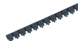
Coding Cover CC-AK1350-GREY Article Number: 51350000000 Is clipped onto the plug from above/on the same side as the screw. The coding cover prevents the AK1350 from being placed on the pin strip 180° off.
