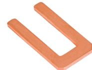
Bridge, 2-pole, BR/2-3.5/3.81-L7.5 Article Number: 50000000015 Uninsulated bridge for multi-connection. Can be used for terminal blocks and multi-connectors with spacing 3.5 mm and 3.81 mm.
