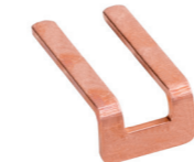
Bridge, 2-pole, angled, BR/2-3.5/3.81-H-L7.5 Article Number: 50000000029 Angled uninsulated bridge for multi-connection. Can be used for terminal blocks and multiconnectors with spacing 3.5 mm and 3.81 mm.
