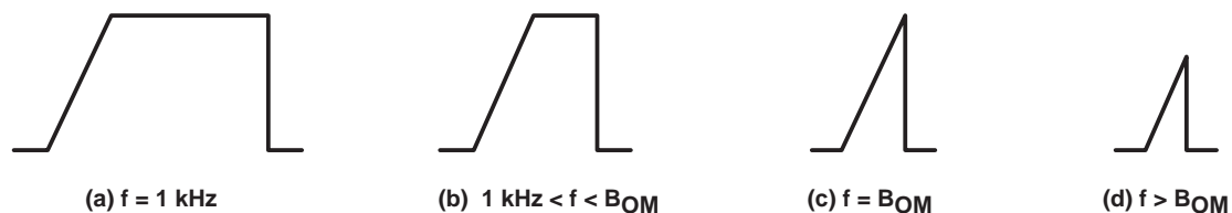
Figure 5. Full-Power-Response Output Signal
